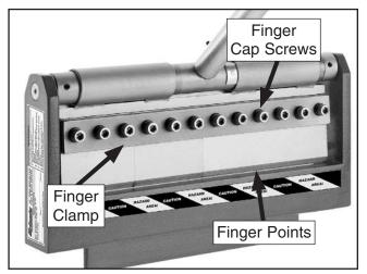
Figure 18. Finger points and cap screws.
